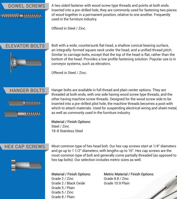
Bolt with a wide, countersunk flat head, a shallow conical bearing surface, an integrally-formed square neck under the head, and a unified thread pitch. Similar to carriage bolts, except that the top of the head is flat, rather than the bottom of the head. Provides a low profile fastening solution. Popular use is in
