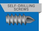
**BSD** - Standard Self Drilling Screw Style; Spaced threads & a drill bit styled point. Eliminates need for pre-drilling. Used for both wood and metal materials.
